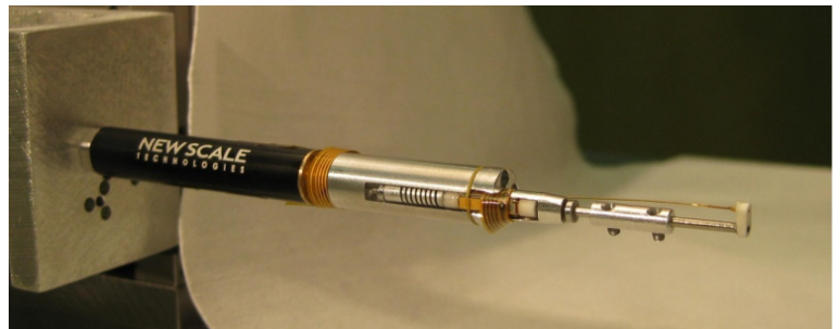
Rigid Fiber Positioners that reconfigure in ~40 sec with 5 \mu\text{m} translational accuracy and no tilt
