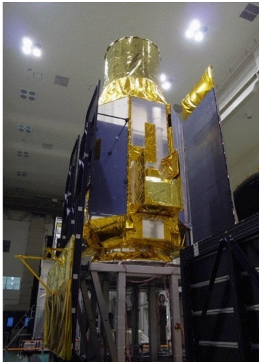
ASTRO-H in JAXA's 13 m thermal-vacuum chamber
