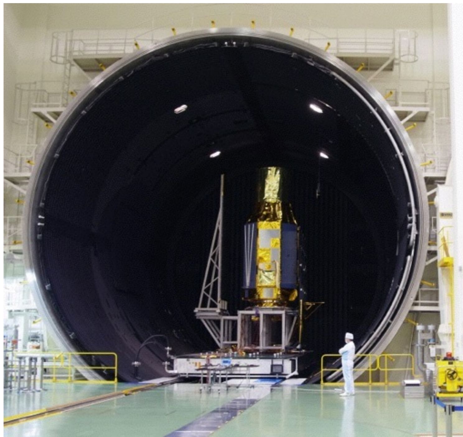
ASTRO-H in JAXA's 13 m thermal-vacuum chamber
