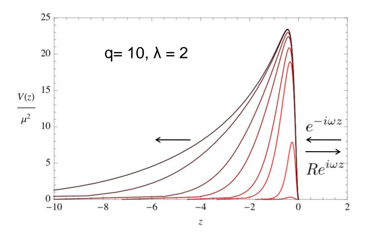
The potential grows as  $T/T_c$  gets smaller. V remains finite at T = 0, so Re  $\sigma(\omega) \neq 0$ . There is no hard gap in the conductivity. (See also Basu, He, Mukherjee, Shieh, 2009)
